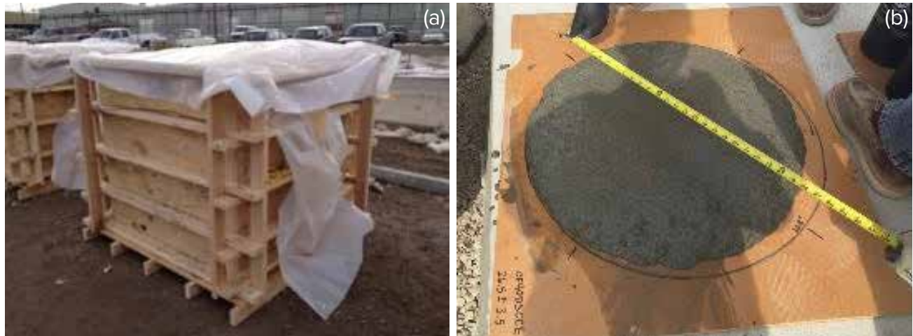
Fig. 2.14.6: Mass concrete placements typically require extensive testing programs, including: (a) instrumentation of large mockups to evaluate heat build-up; and (b) development of SCC mixtures. (Images courtesy of Kiewit Corporation.)
