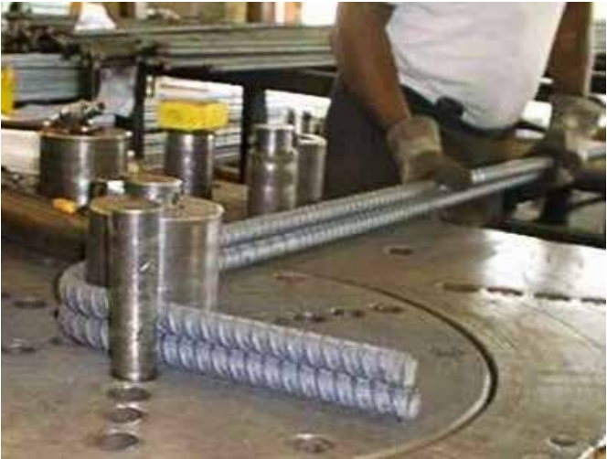
Fig. 2.7.9: A worker uses a bar bender to fabricate standard 90-degree hooks on two No. 9 bars. (Image courtesy of CRSI.)
