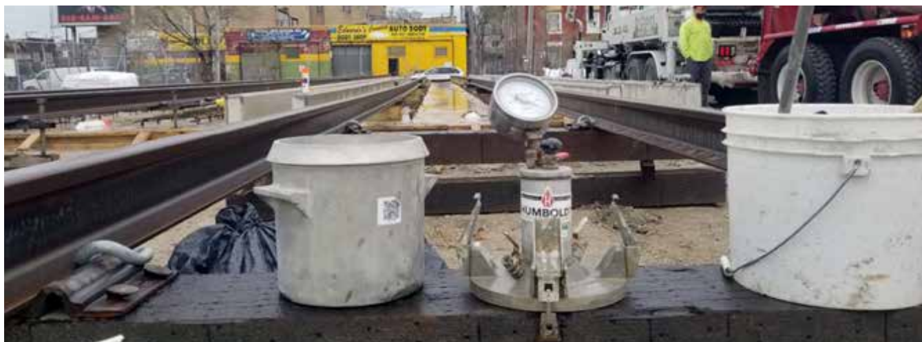
Fig. 2.13.1: Concrete tests include evaluations of air content. (Image courtesy of Flood Testing Laboratories, Inc.)
