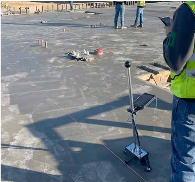
Fig. 2.8.4: Floor flatness ( F_F ) and floor levelness ( F_L ) testing is conducted within 72 hours after concrete placement and before shoring of supported slabs is released or strands are tensioned in PT slabs. Per ASTM E1155, levelness ( F_L ) is not a standard that is tested on unshored elevated/suspended slabs. (Image courtesy of Hensel Phelps.)
