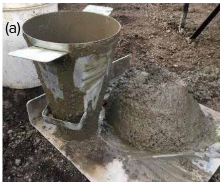
Fig. 2.14.5: Tremie concrete requires mixtures capable of flowing without segregation: (a) example of “bad” concrete mixture approved by client; and (b) examples of “good” concrete mixtures proposed by contractor. (Images courtesy of Kiewit Corporation)
