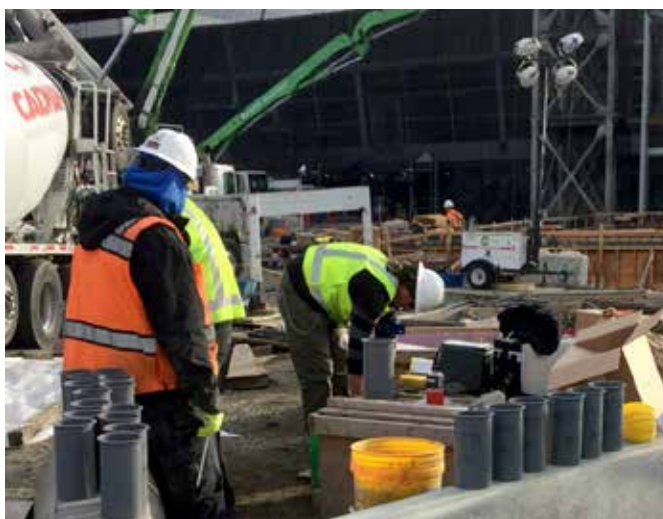
Fig. 2.8.3: Technicians conduct concrete testing (slump and air content) at the point of delivery. (Image courtesy of The Conco Companies.)
