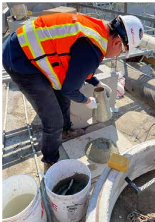
Fig. 2.13.7: A technician conducts a slump test on a formwork deck near the point of placement. (Image courtesy of Ceko Concrete Construction.)
