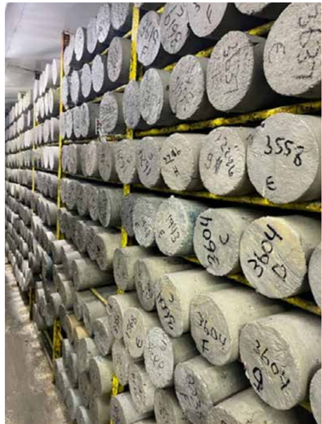
Fig. 2.13.3: A visit to the testing agency's lab should include an inspection of their test cylinder curing room. (Image courtesy of Flood Testing Laboratories, Inc.)
