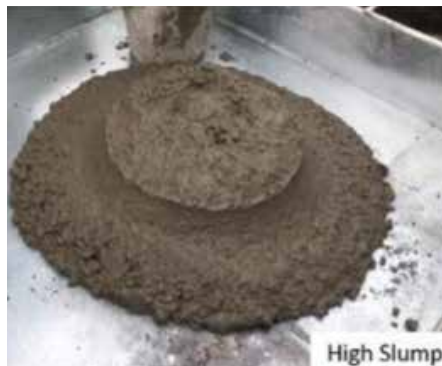
Fig. 2.14.5: Tremie concrete requires mixtures capable of flowing without segregation: (a) example of “bad” concrete mixture approved by client; and (b) examples of “good” concrete mixtures proposed by contractor. (Images courtesy of Kiewit Corporation)
