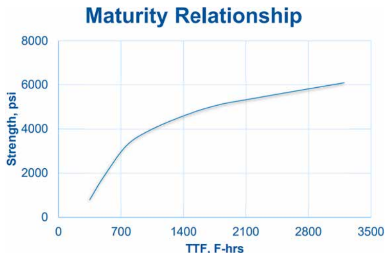
Fig. 2.13.6: The testing agency develops the relationship between compressive strength and temperature-time factor (TTF) for a concrete mixture similar to those that will be evaluated on the project. (Image courtesy of Flood Testing Laboratories, Inc.)
